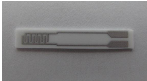
Fig. 1. Ceramic body with platinum electrodes.
