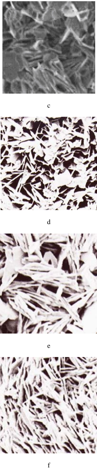
Fig. 5. SEM micrographs at 1000 x (a) Sample quenched from 1200 °C, (b) Sample quenched from 1250 °C, (c) Sample quenched from 1300 °C. (d) Sample quenched on brass, (e) Sample quenched on steel, (f) Sample quenched on copper.
