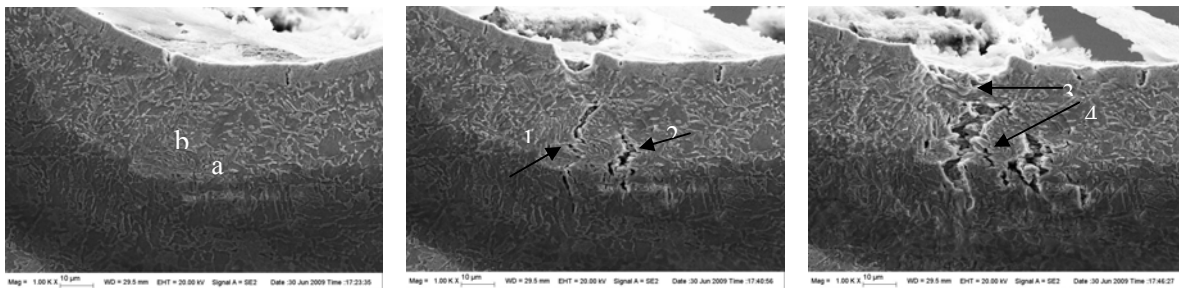
Fig. 8. Micro-crack formation and cracks extension picture of in-situ SEM specimen.
