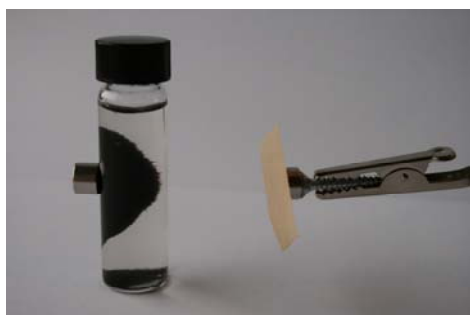
Fig. 4. Magnetic responsiveness of magnetic nanoparticles used for electrospun of nanofibres as well as final fabric can be easily illustrated using small NdFeB magnets.
