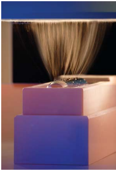
Fig. 1. Magnetically responsive nanofibres were prepared using recently developed Nanospider™ technology. Above, the whole equipment is shown and underneath is the detail on the jet of electrospun nanofibres.
