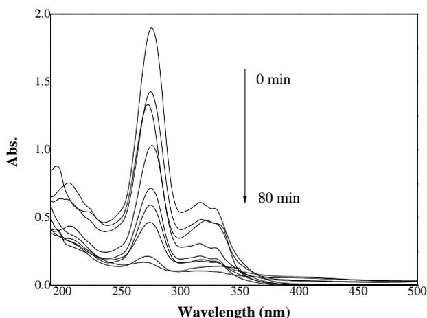
Fig. 4. UV-vis absorption of CPLX with the variation of irradiation time under visible light
