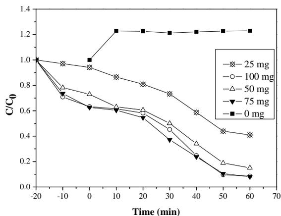
Fig. 5. Photocatalytic degradation of CPLX by CdS with different mass under visible light irradiation.
