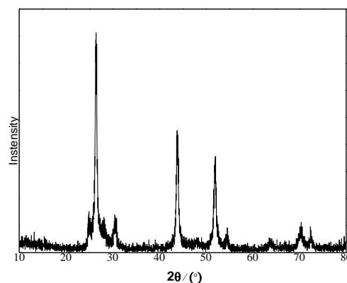
Fig. 2. The XRD spectra of as-prepared CdS photocatalyst
