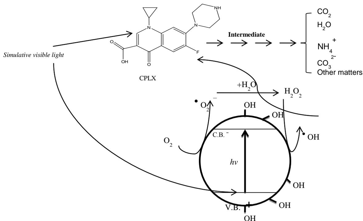
Fig. 6. The schematic diagram of the photocatalytic degradation CPLX with as-prepared CdS under visible light irradiation
