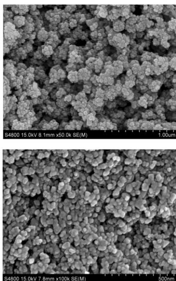
Fig. 1. The FESEM of the as-prepared CdS photocatalyst
