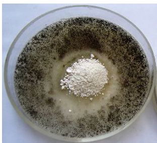
Fig. 7. The aspect of the ZnO powder, after 14 days from inoculation.
