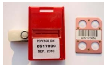
Fig. 1. Albedo dosimeter system used at Dozimed personal Monitoring Service.
