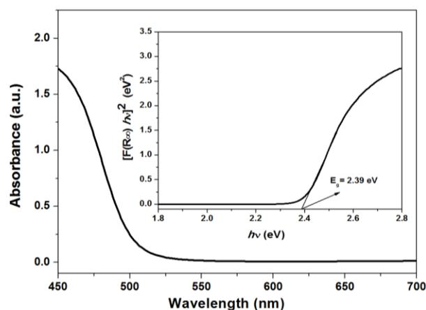
Fig. 6. The variation of absorption coefficient with wavelength and insert shows the corresponding energy band gap ( $E_g$ ) of the PdS/Zn<sub>0.2</sub>Cd<sub>0.8</sub>S photocatalyst
