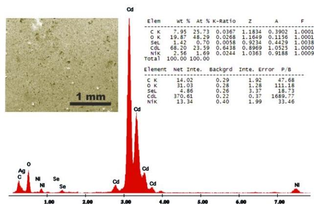
Fig. 2. EDX spectrum of recovered Cd waste from Ni-Cd batteries (insets: left- SEM image of surface used for EDX; right - quantification of elemental composition)
