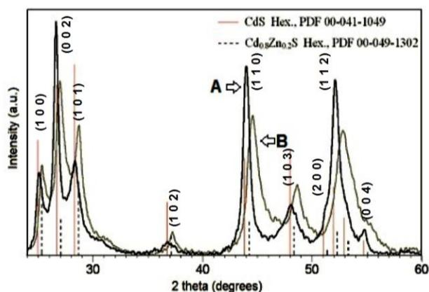
Fig. 3. Comparative XRD profiles for photocatalysts type Zn<sub>0.04</sub>Cd<sub>0.96</sub>S (A) and type Zn<sub>0.2</sub>Cd<sub>0.8</sub>S (B)
