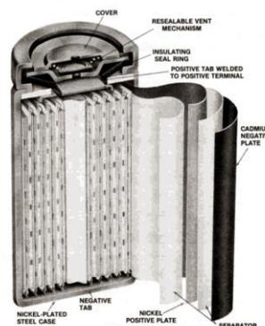
Fig. 1. Ni-Cd battery (section view) [11]
