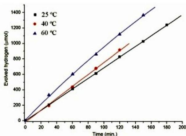
Fig. 7. Hydrogen evolution rate on photocatalyst type  $0.2\%PdS/Zn_{0.2}Cd_{0.8}S$  suspended in  $0.5M Na_2S + 0.25M Na_2SO_3$  aqueous solution, at 25, 40 and 60°C, using simulated AM1.5 solar light illumination
