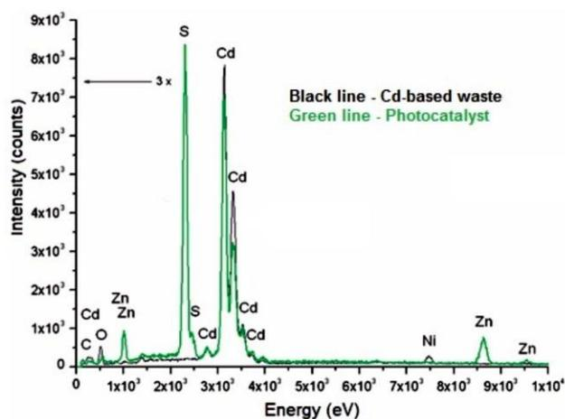
Fig. 5. EDX spectra for cadmium-based waste (black line) and Zn<sub>0.2</sub>Cd<sub>0.8</sub>S-type photocatalyst (green line)
