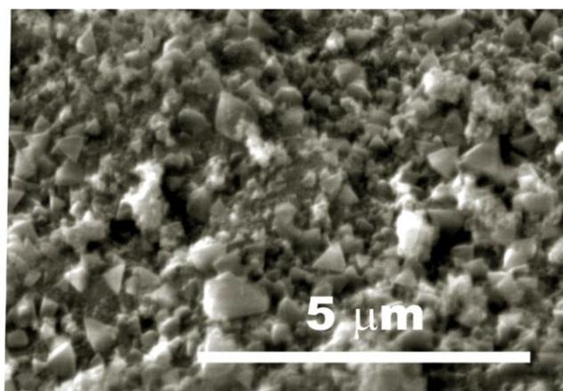
Fig. 4. SEM image of the Zn<sub>0.2</sub>Cd<sub>0.8</sub>S-type photocatalyst
