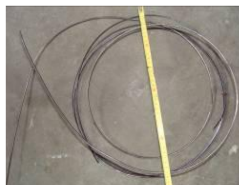
Fig. 2. Magnetic material wire made by Cr-Ni-Fe alloy.
