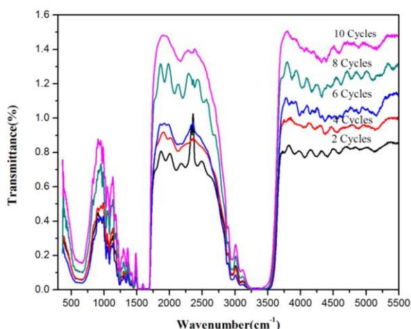
Fig. 2. FT-IR transmission spectrum of CdS-polymer nanocomposites prepared at different cycles of SILAR
