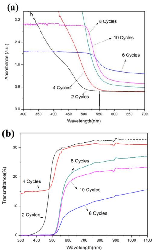
Fig. 1. (a) and (b): Optical absorption and transmission spectrum of CdS-polymer nanocomposites prepared at different cycles of SILAR
