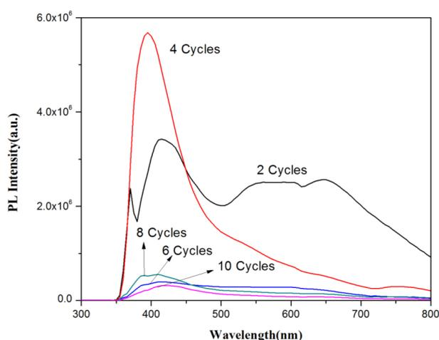
Fig. 3. PL spectrum of CdS-polymer nanocomposites prepared at different cycles of SILAR
