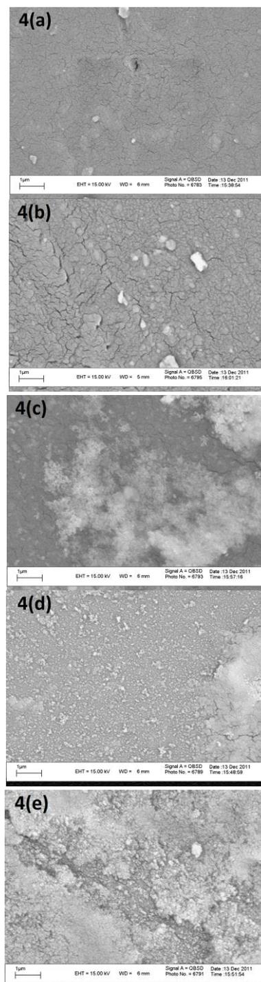
Fig. 4. SEM images of CdS-polymer nanocomposites prepared at different cycles of SILAR, 4(a): 2 cycles, 4(b): 4 cycles, 4(c): 6 cycles, 4(d): 8 cycles and 4(e): 10 cycles
