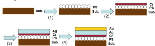
Fig. 3. Schematic illustration of hybrid Au-Ag nanoparticle array fabrication with the following four steps: (1) drop-coating of monolayered PS nanospheres on substrate; (2) deposition of a thin buffer layer of Cr film over the as-coated monolayered PS nanospheres; (3) a further deposition of a layer of Ag film following the Cr deposition; (4) final deposition of a capped layer of Au thin film on top of the Ag film.
