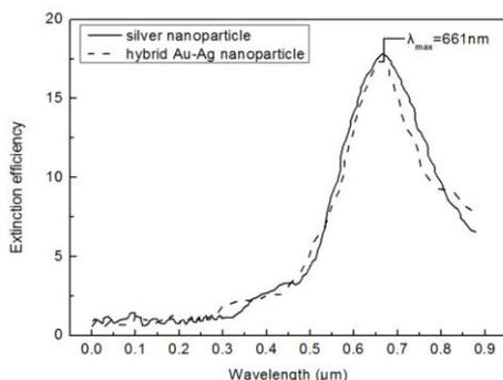
Fig. 6. UV-vis spectra of pure silver nanoparticle arrays (sample a) and hybrid Au-Ag nanoparticle arrays (sample b).
