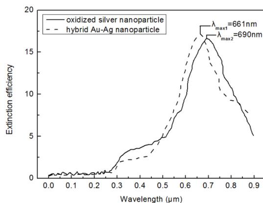
Fig. 7. UV-vis spectra of pure silver nanoparticle arrays (sample a) and hybrid Au-Ag nanoparticle arrays (sample b) exposed to air.
