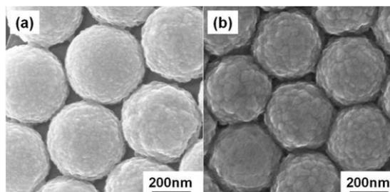
Fig. 9. Representative SEM images of the gas interspaces among the PS spheres deposited with different thicknesses of films: (a) 40 nm; (b) 45 nm.
