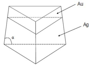
Fig. 1. Schematic illustration of the hybrid Au-Ag triangular nanoparticle arrays in the DDA simulation.
