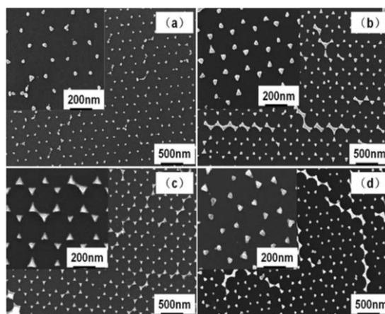
Fig. 8. The SEM images of hybrid Au-Ag nanoparticle arrays for different thicknesses (a) 30 nm; (b) 35 nm; (c) 40 nm and (d) 45 nm.
