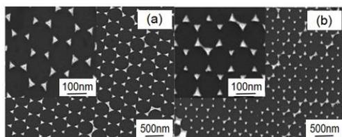
Fig. 5. The SEM images of (a) pure silver nanoparticle arrays and (b) hybrid Au-Ag nanoparticle arrays.
