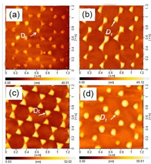
Fig. 10. AFM images of the hybrid Au-Ag nanoparticle arrays for different thicknesses: (a) 30nm; (b) 35nm; (c) 40nm; (d) 45nm.
