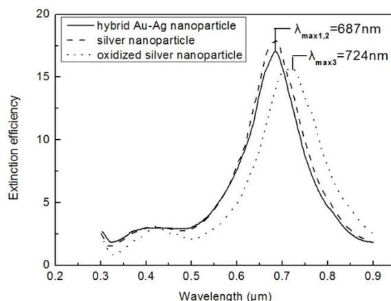
Fig. 4. Calculated spectra of arrays of (Dash) pure silver nanoparticle and (Solid) hybrid Au-Ag nanoparticle and (Dot) silver nanoparticle coated by silver oxide layer.
