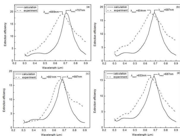
Figs. 11(a)-11(d). Experimental and the calculated extinction spectras of hybrid Au-Ag nanoparticle arrays for different thicknesses: (a) 30 nm; (b) 35 nm; (c) 40 nm and (d) 45 nm.
