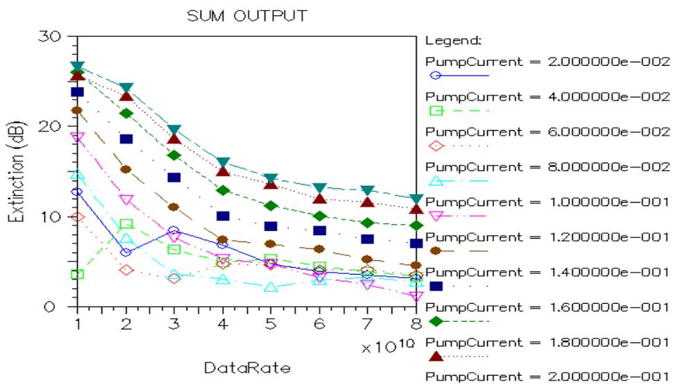
Fig. 10. Extinction vs. data rate vs. pump current
