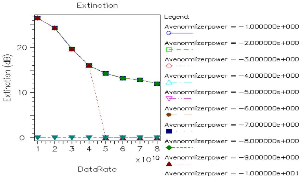
Fig. 15. Extinction vs. data rate vs. Average normalizer power
