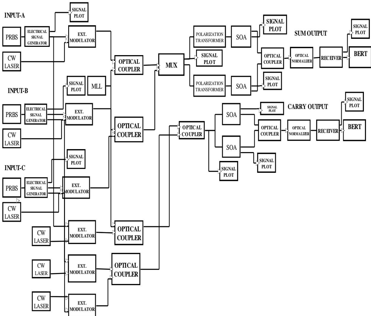
Fig. 1(a). The Full Adder Design
