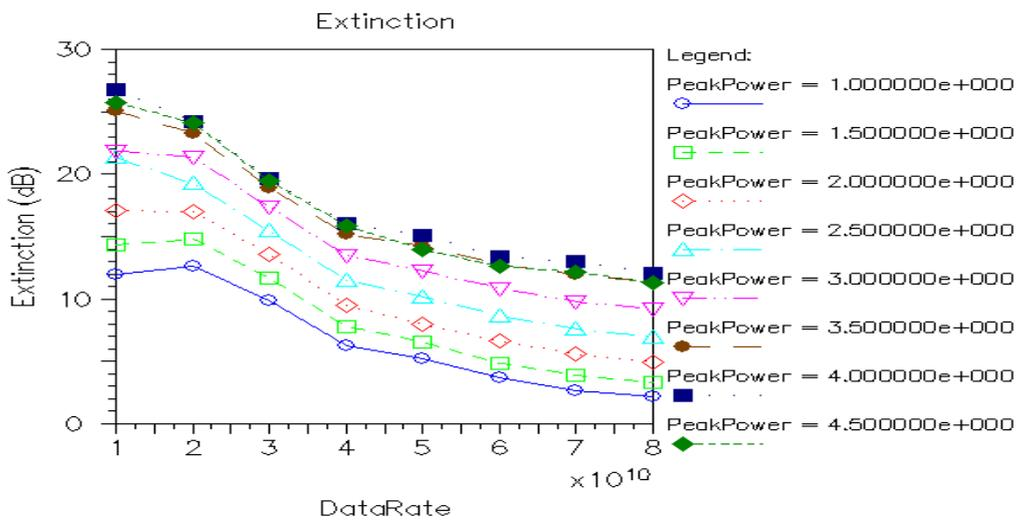
Fig. 8. Extinction vs. data rate vs. probe laser peak power
