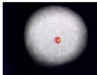
Fig. 1. Chalcogenide lenslet prepared according to the procedure from [14].
