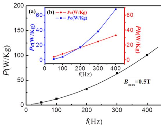
Fig. 5. Dynamic magnetic properties of  $\text{Fe/SiO}_2\text{-Na}_2\text{O-CaO}$  composites at the induction ( $B_{\max}$ ) level of 0.5 T. (a) The core loss ( $P$ ) versus frequency ( $f$ ) curve and (b) Hysteresis loss and eddy current loss of  $\text{Fe/SiO}_2\text{-Na}_2\text{O-CaO}$  composites at different frequencies.
