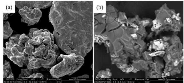
Fig. 1. Representative microstructure of iron powders (a) without and (b) with  $\text{SiO}_2$ - $\text{Na}_2\text{O}$ - $\text{CaO}$  coating.
