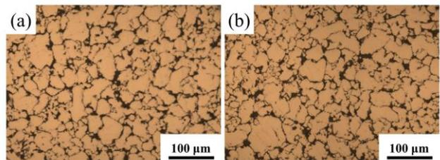
Fig. 2. Representative microstructure of  $\text{Fe}/\text{SiO}_2$ - $\text{Na}_2\text{O}$ - $\text{CaO}$  composites in (a) transverse and (b) longitudinal directions.
