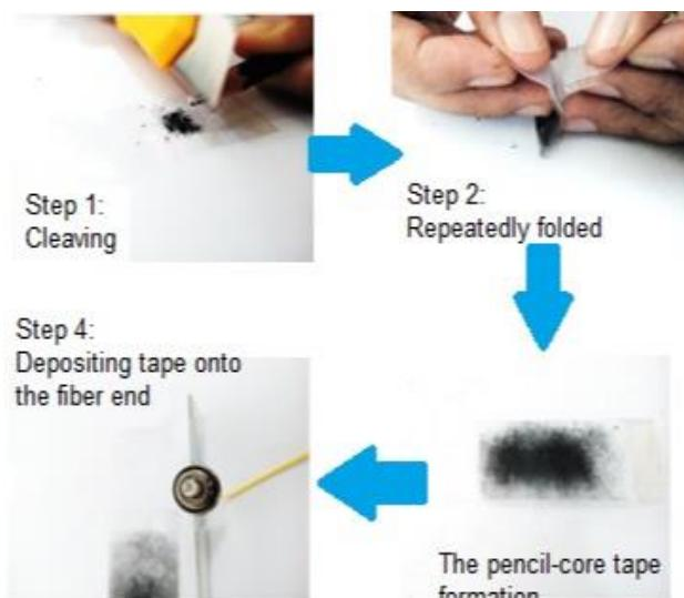
Fig. 1. Simple fabrication process of pencil-core tape
