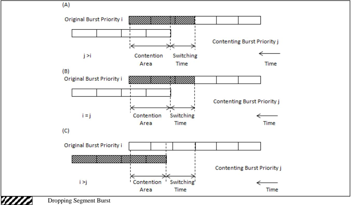
Fig. 2. Reported drop policy in core node (A) Contention of low-priority burst with high-priority burst. (B) Contention of equal priority bursts. (C) Contention of high-priority burst with low-priority burst [7]
