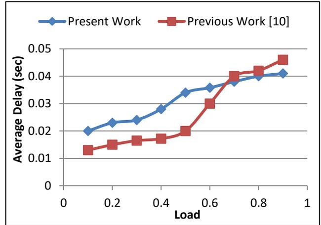
Fig. 9. End to end delay for non-critical traffic at load of 0.2 critical traffic (color online)
