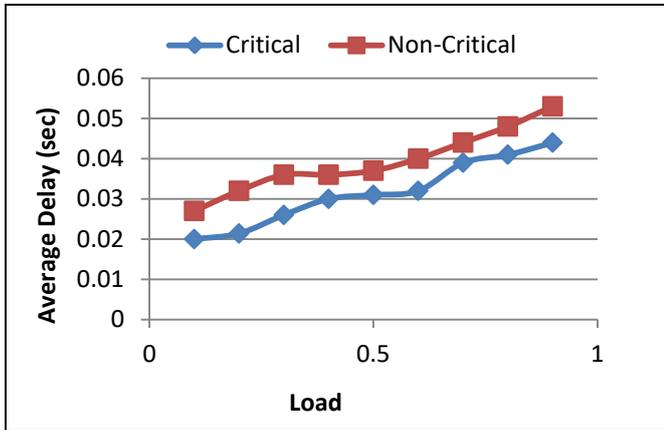
Fig. 7. End to end delay for both critical and non-critical traffic (color online)
