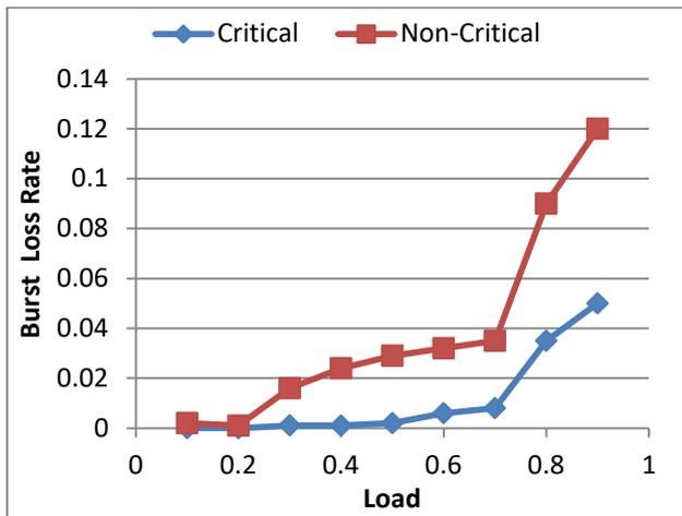
Fig. 4. BLR for both critical and non-critical traffic at equal load (color online)
