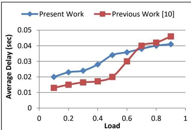
Fig. 8. End to end delay for critical traffic at load of 0.2 non-critical traffic (color online)
