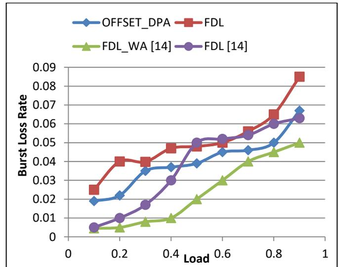
Fig. 6. BLR for non-critical traffic at load of 0.2 for critical traffic. The red and blue symbols are obtained by our design and the violet and green symbols are obtained by Ref. [14] (color online)
