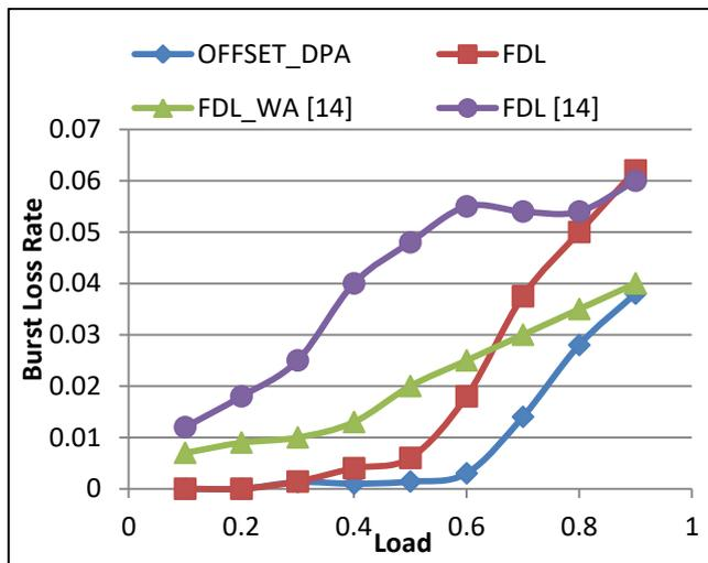
Fig. 5. BLR for critical traffic at load of 0.2 for non-critical traffic. The red and blue symbols are obtained by our design and the violet and green symbols are obtained by Ref. [14] (color online)
