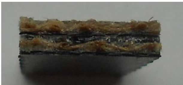
Fig. 1b. Cross-section through hybrid carbon-hemp composite panel.
