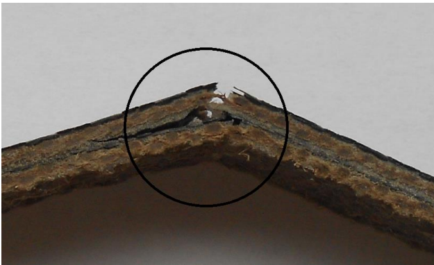
Fig. 10. Side view of carbon-hemp fabric based specimens' break area.
