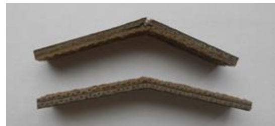
Fig. 2b. Carbon-hemp specimens after bending tests.
