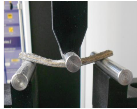
Fig. 2a. Carbon-hemp specimen during three-point bending test.
