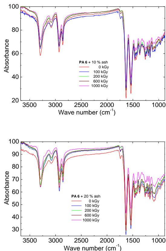
Fig. 2. Spectral modifications in PA 6 modified with rice husk ash in two concentrations after electron beam irradiation at various doses.
