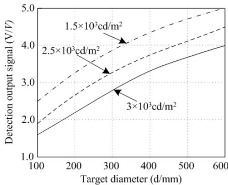
Fig. 4. The changing curve of detection output signal and target diameter under different background luminance
