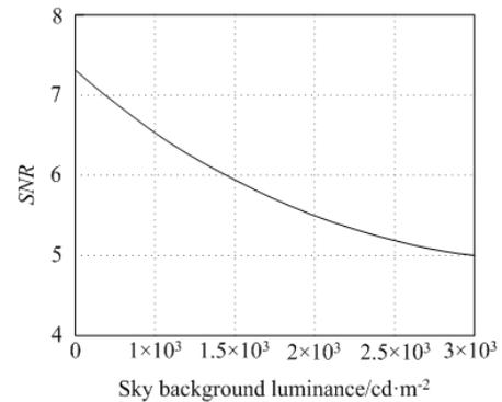
Fig. 3. The change curves of SNR under different sky background luminance
