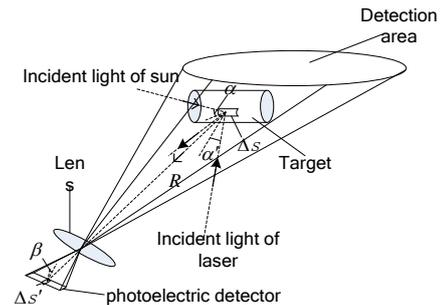
Fig. 2. The space target image principle in photoelectric detection system
