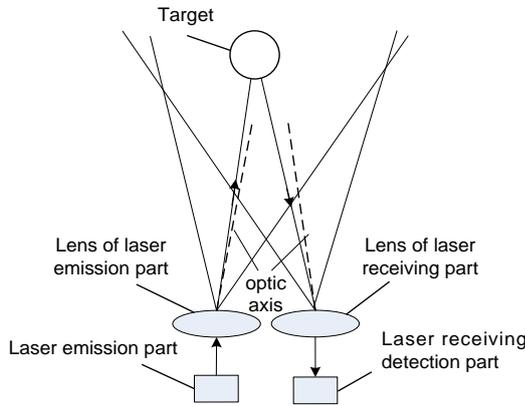
Fig. 1. The detection schematic diagram of laser detection system on space target
