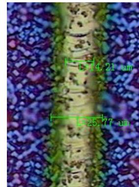
Fig. 9c. Laser scanning microscope images of cells with 100nm  $\text{SiO}_2(\text{B})$  after laser doping
