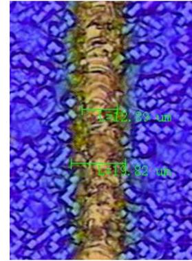
Fig. 9a. Laser scanning microscope images of cells with 400nm  $\text{SiO}_2(\text{B})$  after laser doping
