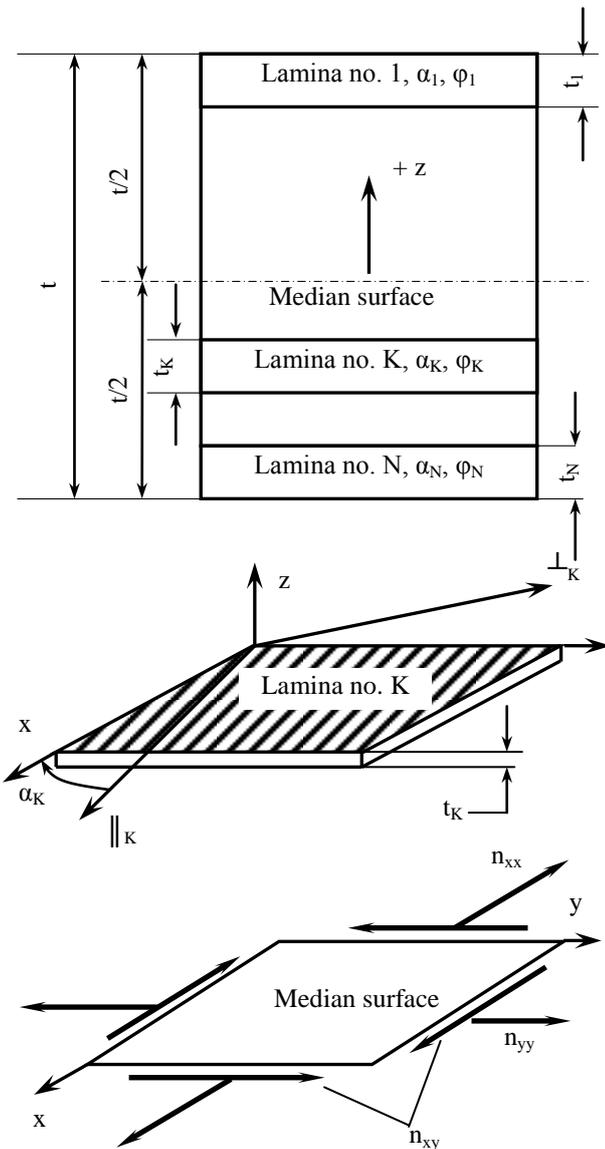
Fig. 1. Constructive scheme of a composite laminate.
