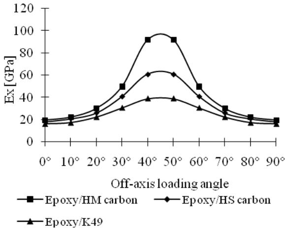
Fig. 7.  $E_x$  Young modulus for a [45/-45/45/-45] epoxy based composite laminate.
