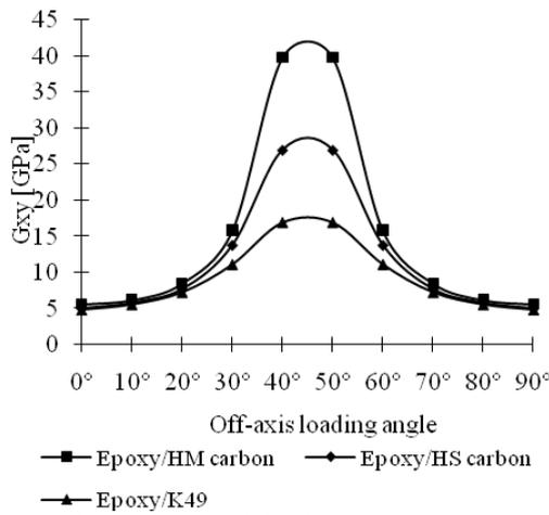
Fig. 2.  $G_{xy}$  shear modulus for a [0/90/0/90] epoxy based composite laminate.
