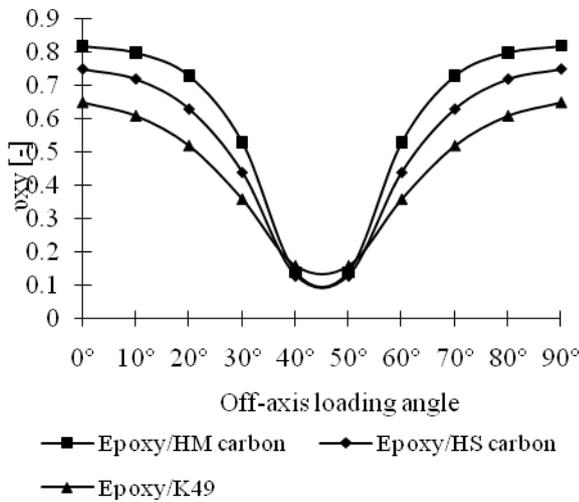
Fig. 9.  $\nu_{xy}$  Poisson ratio for a [45/-45/45/-45] epoxy based composite laminate.
