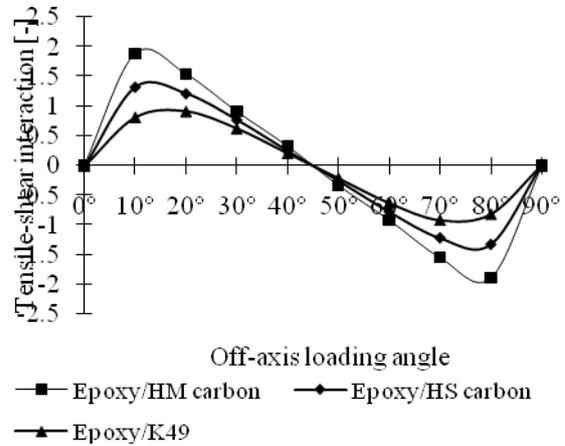
Fig. 15. Distribution of tensile-shear interaction in a [0/90/0/90] composite laminate.
