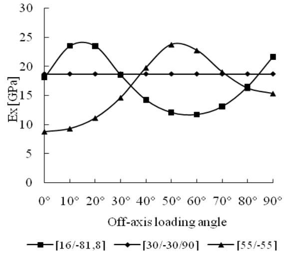
Fig. 10.  $E_x$  Young modulus of three epoxy based glass-fibres composite laminates.
