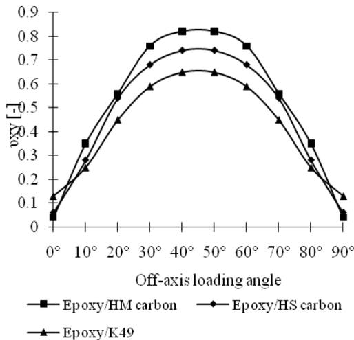
Fig. 3.  $v_{xy}$  Poisson ratio for a [0/90/0/90] epoxy based composite laminate.
