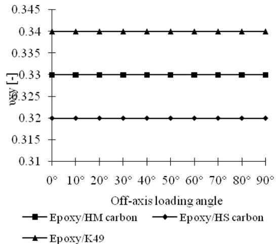
Fig. 6.  $v_{xy}$  Poisson ratio for a [0/45/-45/90] epoxy based composite laminate.
