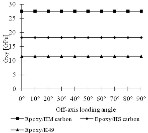
Fig. 5.  $G_{xy}$  shear modulus for a [0/45/-45/90] epoxy based composite laminate.
