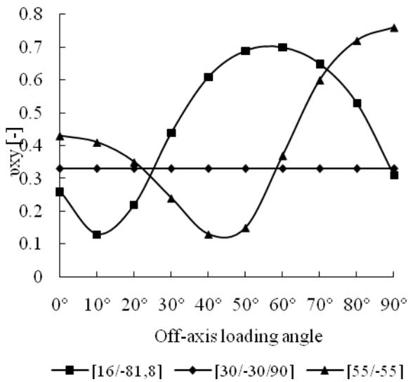
Fig. 13. Poisson ratio distribution of three epoxy based glass-fibres composite laminates.
