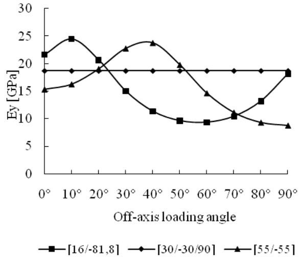
Fig. 11.  $E_y$  Young's modulus of three epoxy based glass-fibres composite laminates.
