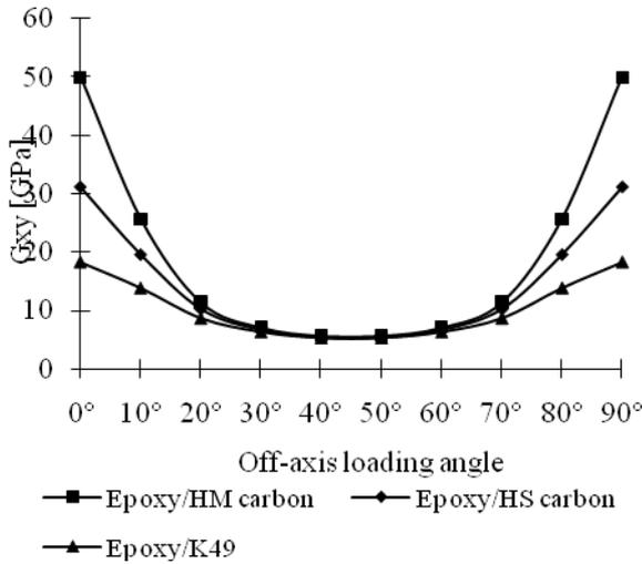
Fig. 8.  $G_{xy}$  shear modulus for a [45/-45/45/-45] epoxy based composite laminate.
