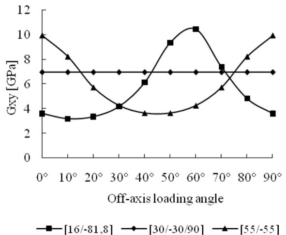
Fig. 12. Shear modulus distribution of three epoxy based glass-fibres composite laminates.
