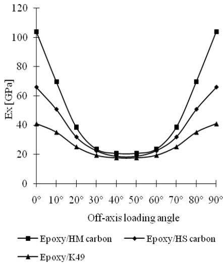
Fig. 1.  $E_x$  Young modulus for a [0/90/0/90] epoxy based composite laminate.
