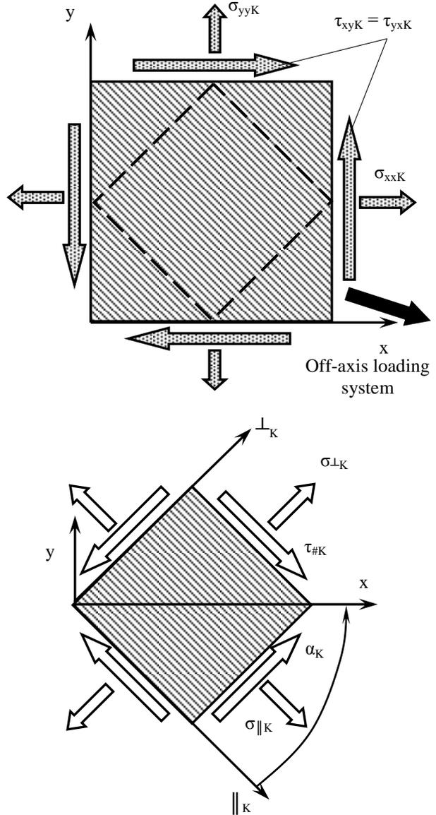
Fig. 2. Loading scheme of a composite laminate.
