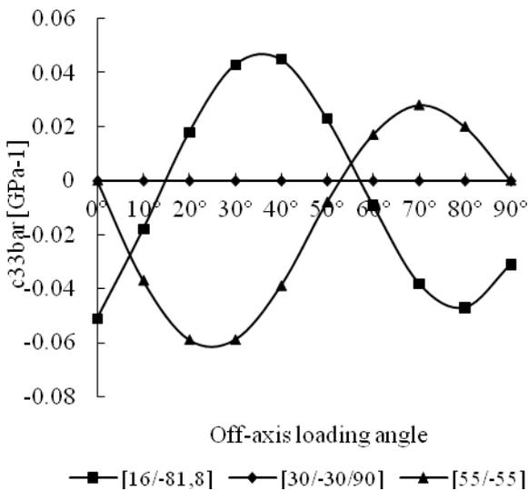
Fig. 14. Distribution of  $\epsilon_{33}$  compound of the transformed compliance tensor.
