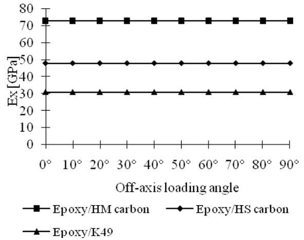
Fig. 4.  $E_x$  Young modulus for a [0/45/-45/90] epoxy based composite laminate.
