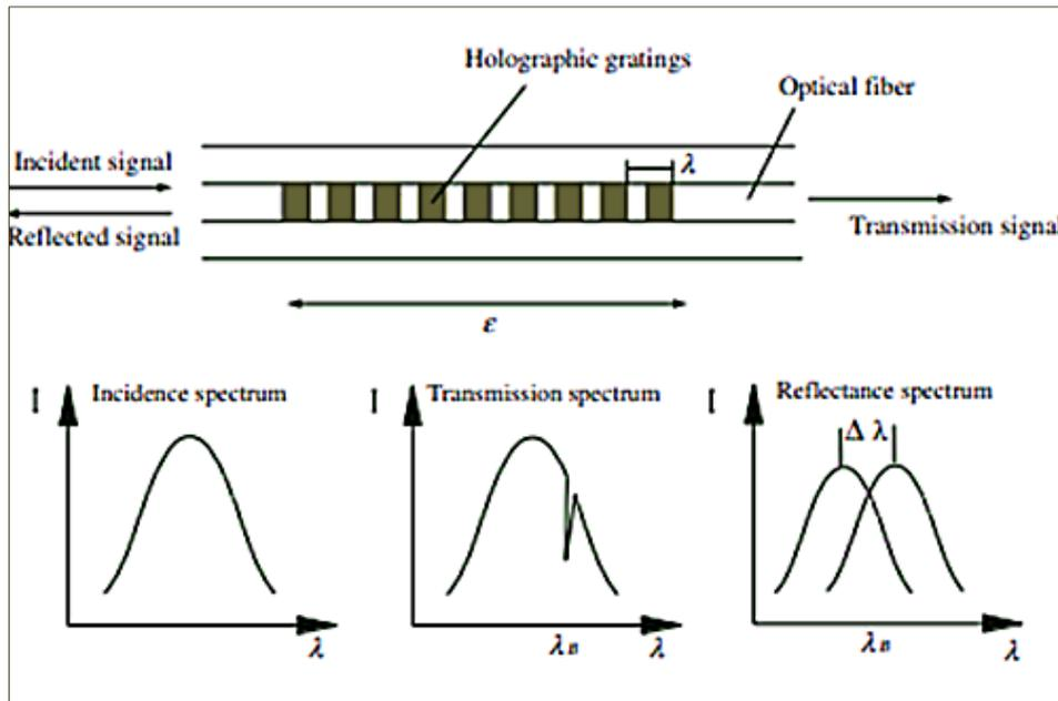
Fig. 1. Schematic diagram of FBG sensing principle
