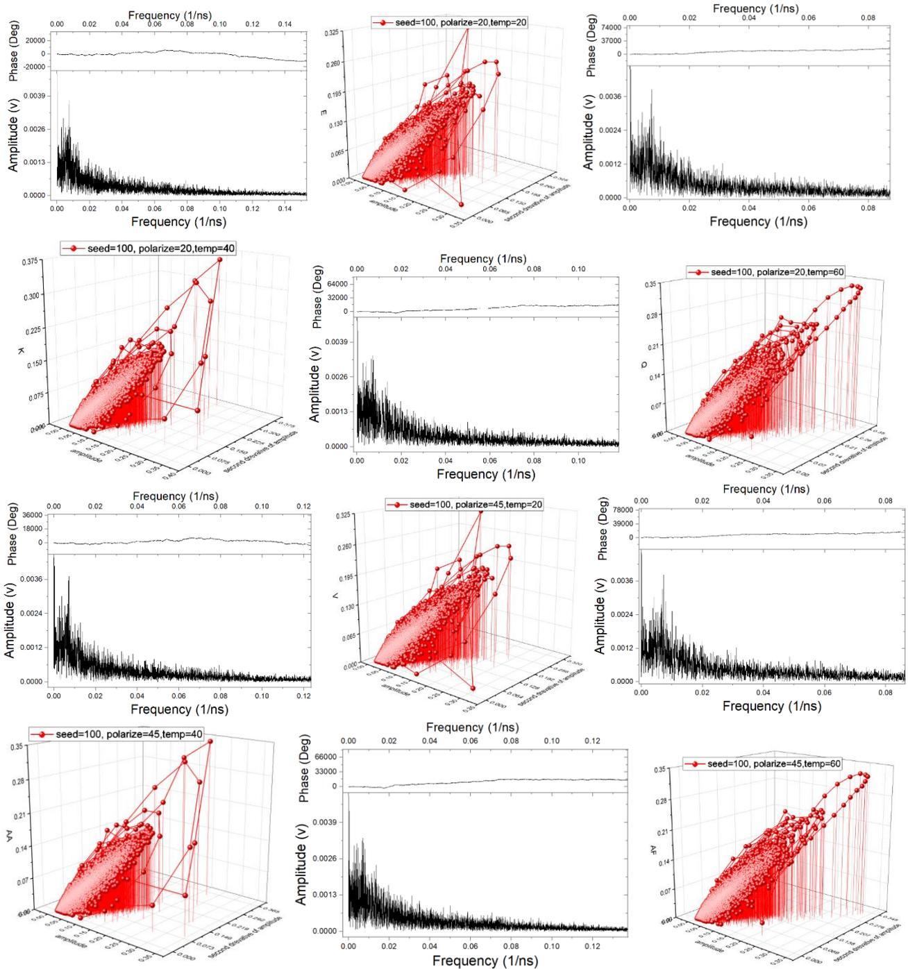
Fig. 6. Results for chaotic output mixed signal combined from LD1 and LD2 with three FBG applied temperatures (20,40,60) °C, and variable polarization. Upper row: FFTs and 3D attractors with SEED 100 and 200 for LD1 and LD2 and polarization 20. Lower row: The same SEEDs as previous part, but with polarization 45 (color online)
