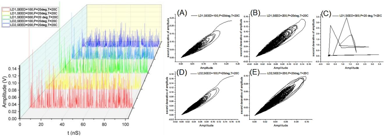
Fig. 3. Results for chaotic dynamics associated with LD1 (OV\_1) with variable seed (100, 200, 300), and LD2 (OV\_2) SEED (100, 200), with constant temperature  $T$  ( $20^{\circ}\text{C}$ ) and polarization  $P$  ( $20\text{ deg.}$ ). (left) Time series (right) Phase space. (A) LD1 SEED (100)  $P(20\text{ deg.})$ , (B) LD1 SEED (200)  $P(20\text{ deg.})$ , (C) LD1 SEED (300)  $P(20\text{ deg.})$ , (D) LD2 SEED (100)  $P(20\text{ deg.})$ , (E) LD2 SEED (200)  $P(20\text{ deg.})$  (color online)
