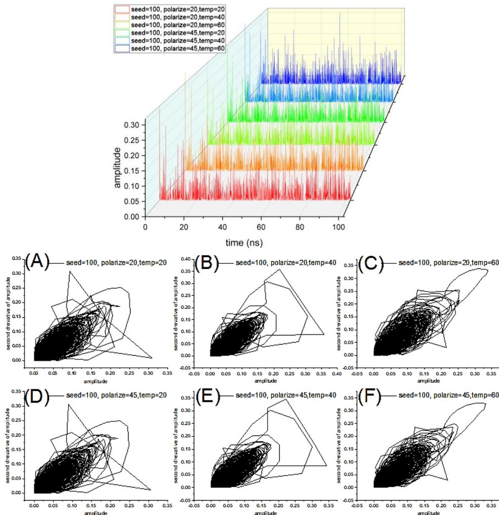
Fig. 5. Results for chaotic output measured time series from OV\_4 for signal mixing between LD1 and LD2, with constant LD1 seed (100) and LD2 seed (200), and variable both  $T$  (20, 40, 60)  $^{\circ}\text{C}$  and  $P$  (20,45) degree (color online)
