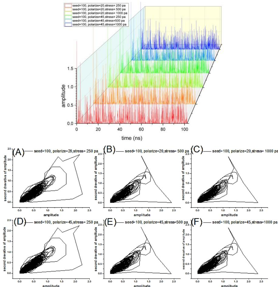
Fig. 7. Results for mixed chaotic output (OV\_4), time series and its attractors with; SEED=100, 200 for LD1 and, respectively. LD1 P is (20,45) deg, FBG sensor T (20) °C, and the applied stress changed with; (250, 500, 1000) MPa (color online)
