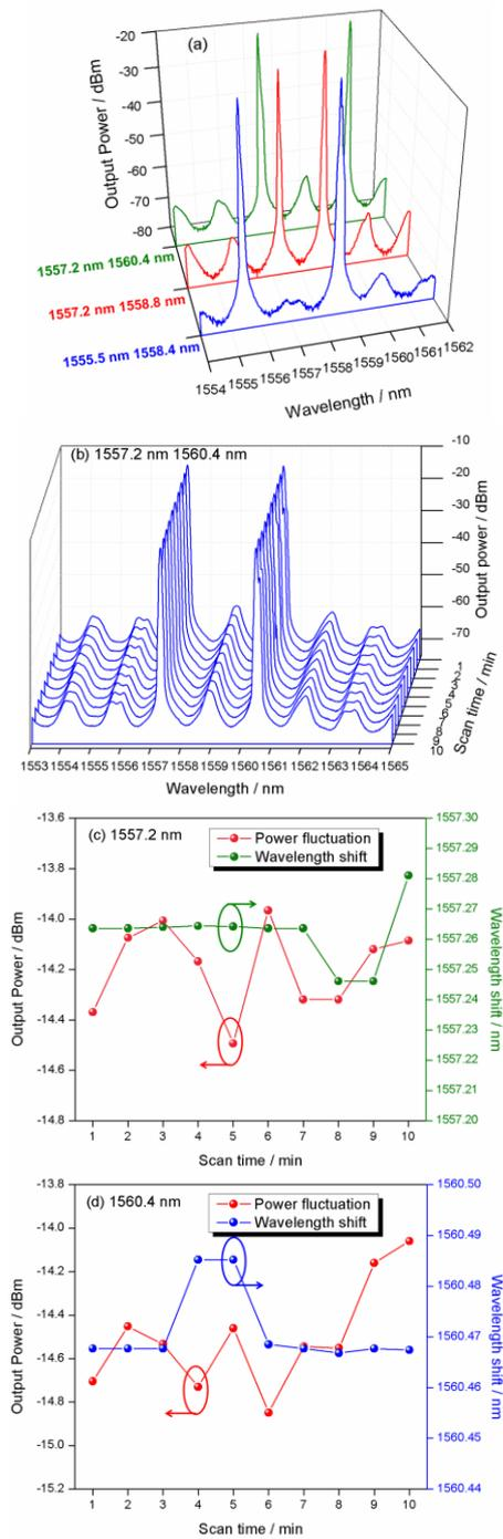
Fig. 7. (a) Tunable double-wavelength laser; (b) spectrum of the double-wavelength laser obtained by scanning for 10 min; (c) stability of the 1557.2 nm laser; (d) stability of the 1560.4 nm laser
