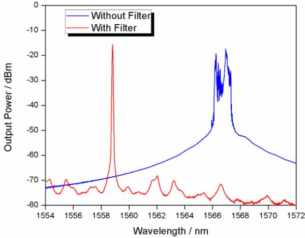
Fig. 4. Laser spectrum before and after using the filter
