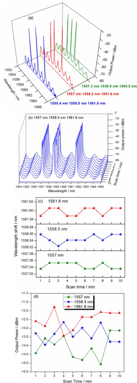
Fig. 8. (a) Tunable triple-wavelength laser; (b) spectrum of the triple-wavelength laser obtained by scanning for 10 min; (c) wavelength stability of the triple-wavelength laser; (d) power stability of the triple-wavelength laser
