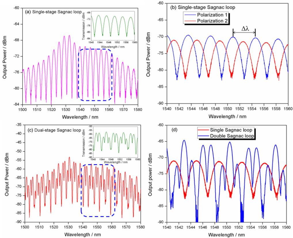
Fig. 3. (a) Transmission spectrum of the single Sagnac loops within 1500–1580 nm; (b) single Sagnac loops within 1540–1560 nm; (c) transmission spectrum of the double Sagnac loops within 1500–1580 nm; (d) double Sagnac loops within 1540–1560 nm
