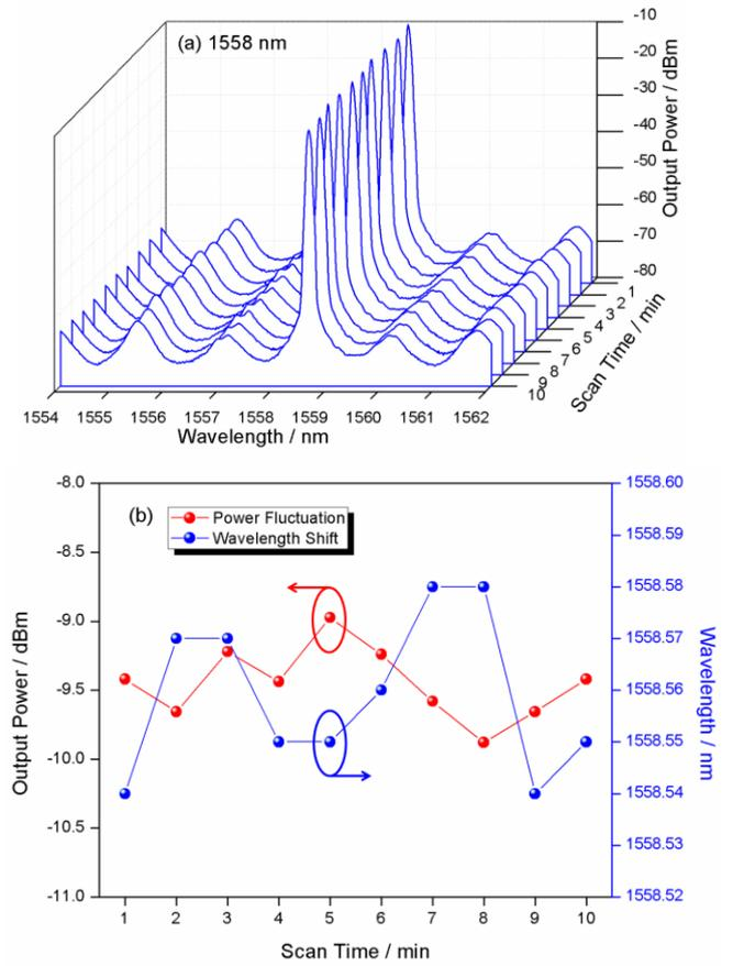
Fig. 6. (a) Scanning spectrum and (b) stability of the 1558 nm laser
