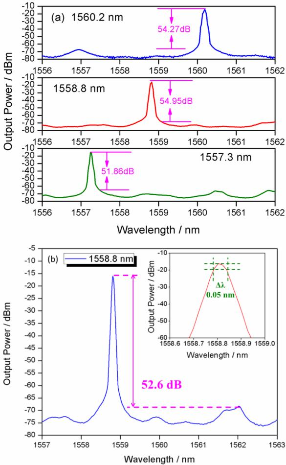
Fig. 5. (a) Single-wavelength tuning ability; (b) spectrum of the 1558.8-nm laser
