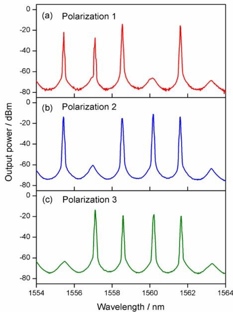
Fig. 9. Tunable quadruple-wavelength laser
