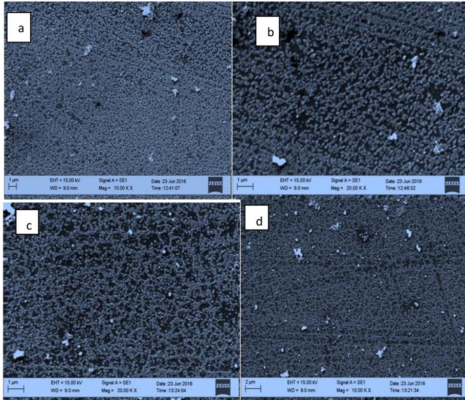
Fig. 3. SEM micrographs of CuInS<sub>2</sub> films (a,b) Un-doped film (c,d) Doped film
