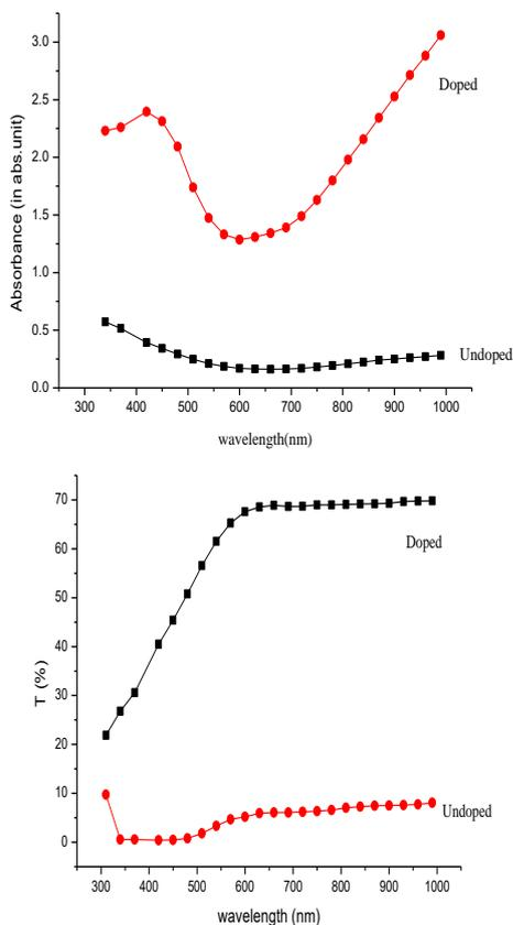
Fig. 5. Absorbance and transmission spectra of doped and un-doped  $\text{CuInS}_2$  films
