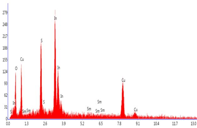
Fig. 4. EDX profile of doped  $\text{CuInS}_2$  film
