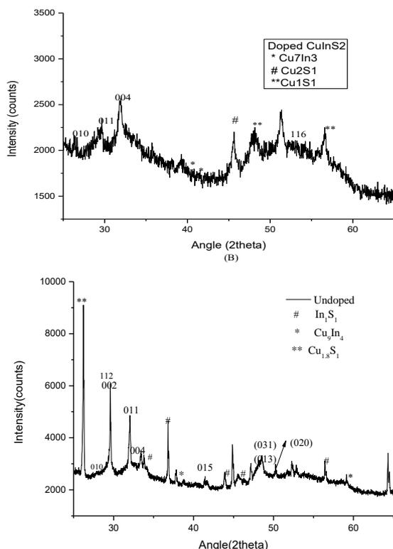
Fig. 1. XRD spectra of un-doped and Sm doped  $\text{CuInS}_2$  thin films
