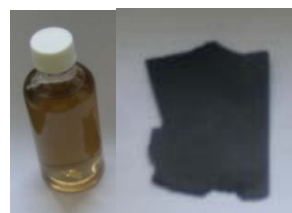
Picture 1. Left –colloidal suspension of graphite oxide and right-graphite oxide paper like.
