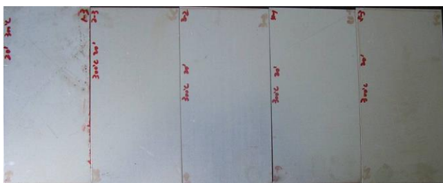
Fig. 12. The appearance of the passivation film after baking at elevated temperature.
