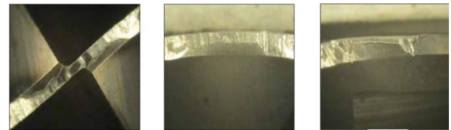
Fig. 13. The second cutting experiment of single gradient AlCrN coating tool edge local fracture morphology.
