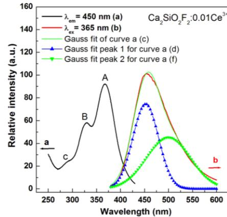
Fig. 2. UV excitation spectrum (a:  $\lambda_{em} = 450$  nm) and emission spectrum (b:  $\lambda_{ex} = 365$  nm) of  $\text{Ca}_2\text{SiO}_2\text{F}_2:0.01\text{Ce}^{3+}$  phosphors
