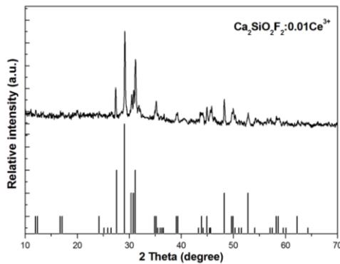
Fig. 1. XRD patterns of sample  $\text{Ca}_2\text{SiO}_2\text{F}_2:0.01\text{Ce}^{3+}$  and the standard pattern of ICSD-19-1131
