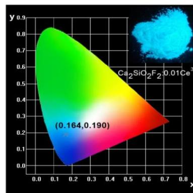
Fig. 5. Color coordinates of  $\text{Ca}_2\text{SiO}_2\text{F}_2:0.01\text{Ce}^{3+}$  in the CIE chromaticity diagram and the inset shows a photograph of the blue-emitting phosphor  $\text{Ca}_2\text{SiO}_2\text{F}_2:0.01\text{Ce}^{3+}$  taken under 365 nm excitation in a UV lamp
