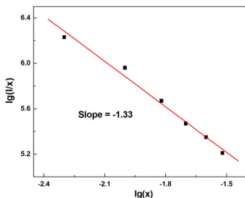
Fig. 4. The curve of  $\lg(x)$  versus  $\lg(I/x)$  of  $\text{Ca}_2\text{SiO}_2\text{F}_2:x\text{Ce}^{3+}$  phosphors
