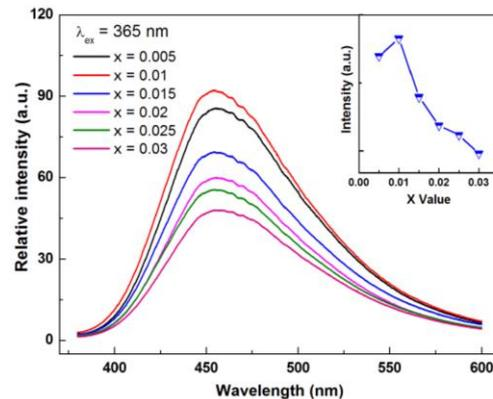
Fig. 3. Emission spectra of  $\text{Ca}_2\text{SiO}_2\text{F}_2:x\text{Ce}^{3+}$  phosphors under 365 nm excitation. The right inset shows the dependence of PL intensity on the  $\text{Ce}^{3+}$  doping concentration ( $x$  value)
