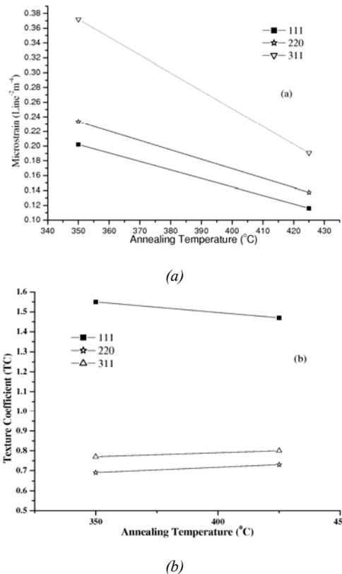
Fig. 2. Variation of micro strain (a) and Texture coefficient (b) for plane (111), (220) and (311) at different annealing temperature.
