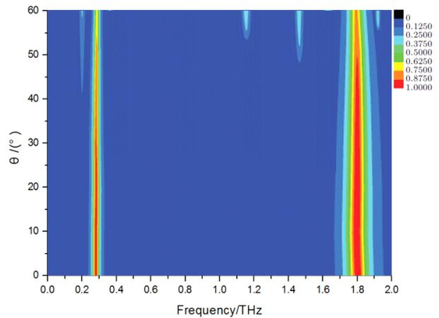
Fig. 7. The change of the absorption with different incident angles under the condition of vertical incidence
