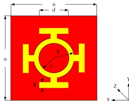
Fig. 1. The structure diagram of the absorber
