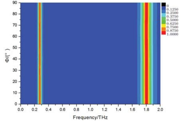
Fig. 6. The change of the absorption peak with different polarization angles under the condition of vertical incidence
