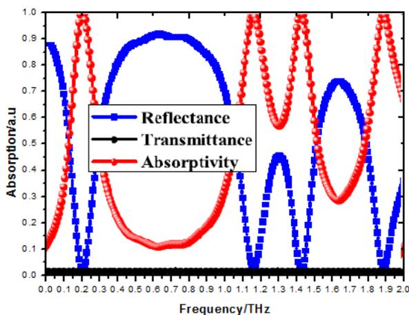
Fig. 2. The reflectance, transmittance and absorptivity of proposed absorber
