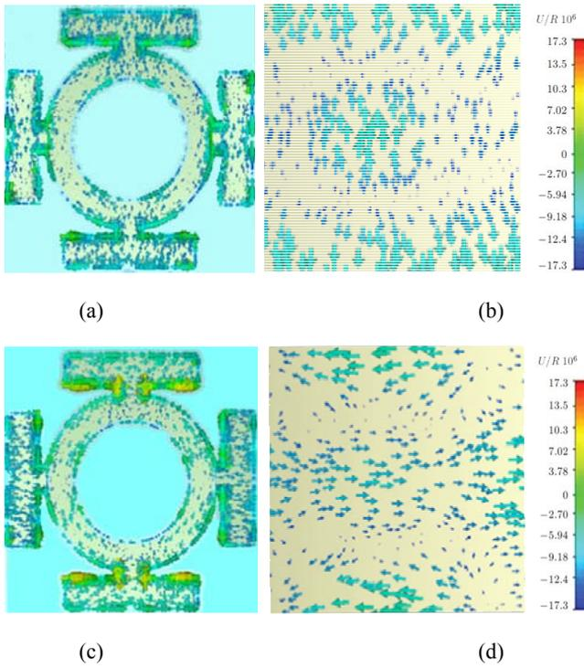
Fig. 4. The surface current and z component of absorber
