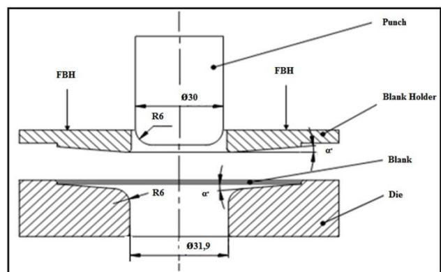
Fig. 2. A new type deep drawing die.
