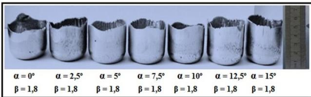
Fig. 4. Relation between  $\beta$  and  $\alpha$  and formation of wrinkles
