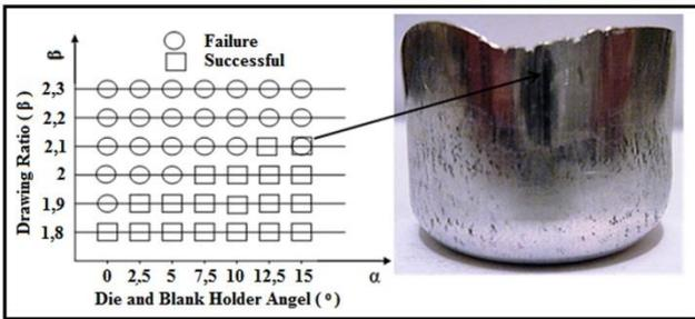
Fig. 3. Relationship between  $\beta$  value and  $\alpha$  angle.
