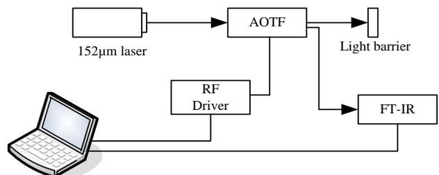
Fig. 3. Setup of experiment for diffraction efficiency of AOTF.
