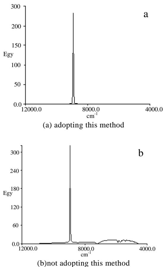
Fig. 4. Effect of rejecting zero order light with orthogonal polarizing method.
