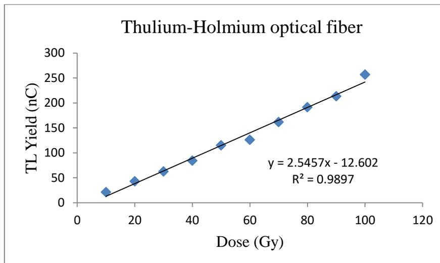
Fig. 1. The TL response of Thulium-holmium doped optical fiber versus dose
