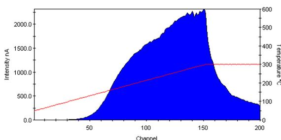
Fig. 2. The glow curve of Thulium-holmium doped  $\text{SiO}_2$  optical fiber for 90 Gy dose of gamma irradiations
