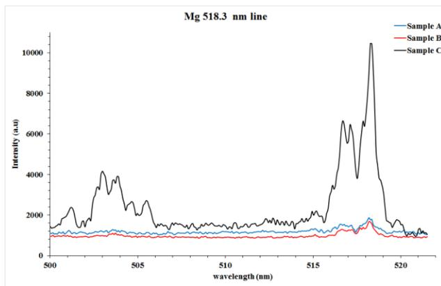
Fig. 8. Comparison of Mg line at 518.3 nm for three samples.
