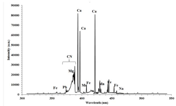
Fig. 5. The LIBS spectrum of the groundwater sample (sampling well B) in the wavelength region of 300nm to about 500 nm. None of the elements of interest appears above that wavelength range for this sample.
