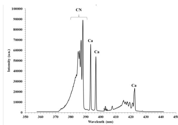
Fig. 3. The LIBS spectrum of the wood slices alone in the wavelength region of 350 nm to 450 nm before the absorption of the liquid samples.
