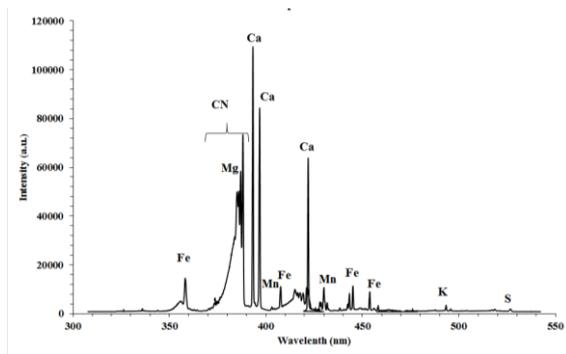
Fig. 4. The LIBS spectrum of the groundwater well (sampling site A) in the wavelength region of 350nm to 550nm.
