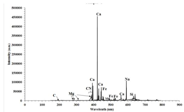
Fig. 6. The LIBS spectrum of the groundwater sample (sampling well C) in the wavelength region of 300nm to 800nm.
