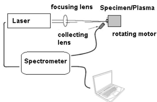
Fig. 3. Schematic representation of the LIBS system used.
