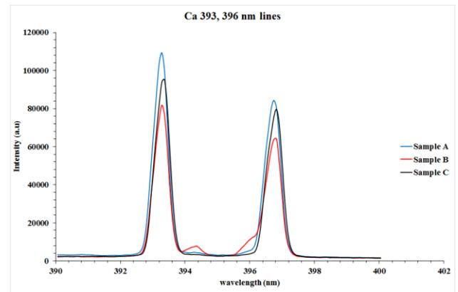
Fig. 10. Comparison of Ca line at 393 & 396 nm for three samples.
