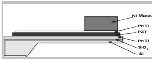
Fig. 8. Schematic configuration of a single cantilever beam [18].
